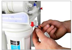
Remove the white plug from the water input adaptor. Pull out the blue clip. Compress white tube sleeve and remove the white plug.
