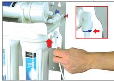
Take the white tube and insert one end of it into the water input adapter. Replace the blue clip from the previous step to lock the tube into place.
