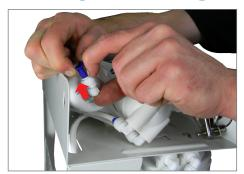
Remove the blue plug from the deionizing filter housing output. Pull out the blue clip. Compress the white tube sleeve and remove the blue plug.
