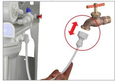
On the other end of the white tube, attach the 3/4 inch faucet adapter. This will thread onto any 3/4 inch faucet spout. This line allows water into the R.O. machine.
