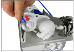
Take the blue tube and insert one end of it into the DI-Filter housing output adapter. Replace the blue clip from the previous step to lock the tube into place.
