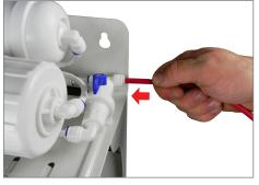
Take the red tube and insert one end of it into the waste water output adapter. Replace the blue clip from the previous step to lock the tube into place.
