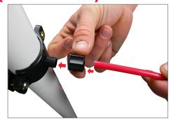
Attach the other end of the red tube to the drain bracket. Run the red tube through the black nut into the drain bracket; tighten down to lock tube into place.
