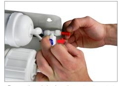
Remove the red plug from the wastewater output adapter. Pull out the blue clip. Compress the white tube sleeve and remove the red plug.
