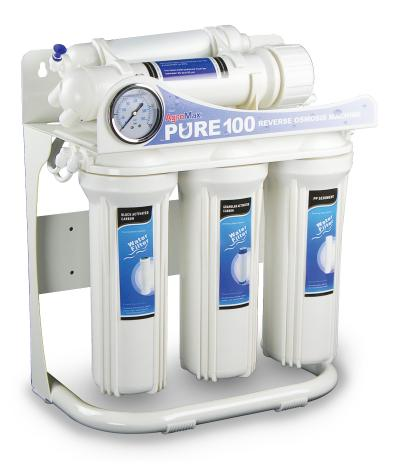
THE R.O. MEMBRANE should be periodically flushed. This will help keep membrane working properly and will significantly extend its life. It is recommended to flush the membranes after every use (or every 100 gallons). This is done by simply flipping on the flush valve located behind the deionizing filter.
