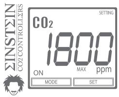
Use the "SET" button to switch between the Minimum Set Point and the Maximum Set Point. Once both values are set to users preference the unit will blink for roughly 10 seconds and the new values will be saved.
