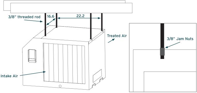
Parts Needed: 4 pieces 3/8" threaded rod (not included) 4 - 3/8" threaded jam nuts (not included)
