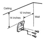
**NOTE:** The bracket should be positioned at least 14 inches from the ceiling and at least 12 inches from adjoining wall.
