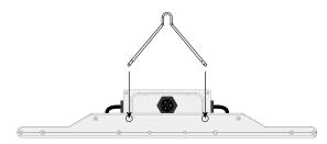
3 • Connect the NextLight Pro Series Power Cord to the AC In on the Driver.
