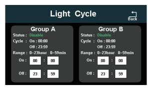
IN Auto mode, set turn on time and turn off time, timing cycle is 24 hours.
